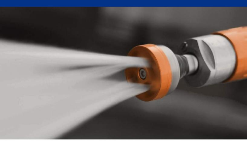
The SCIMITAR H is a robust hydro-jetting tool with rotation control through a centrifugal brake, offering high efficiency. It is specially designed for surface treatment services in manual operations with a gun or in automated processes.
